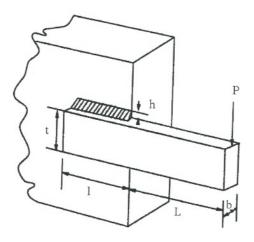
Fig. 2. The welded beam problem
